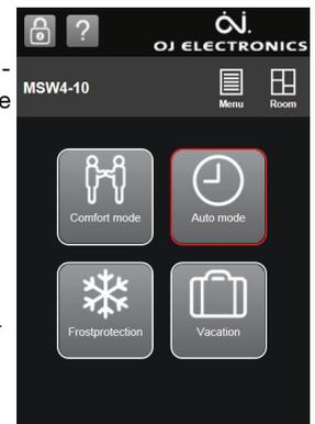
The comfort system is now in Vacation mode and the suitcase is displayed. Once the period has elapsed, the Central Controller will automatically return to **Auto mode**.
